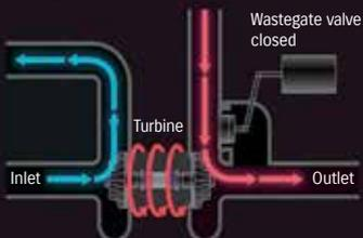
Closed for normal driving, it helps apply higher boost pressure to achieve excellent torque response.
