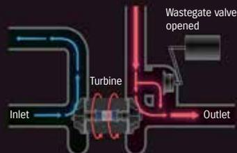
Opened for cruising, it prevents overpressure and suppresses fuel consumption.
